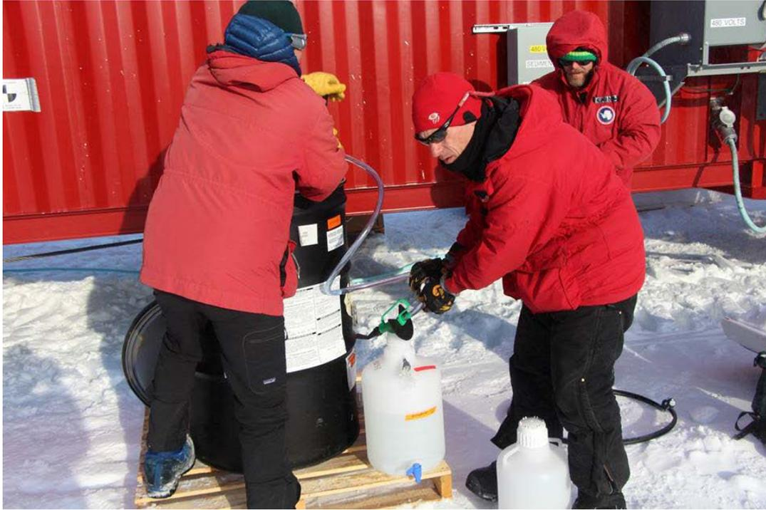
**Preparing hydrogen peroxide solution for cleaning of down borehole tools**
