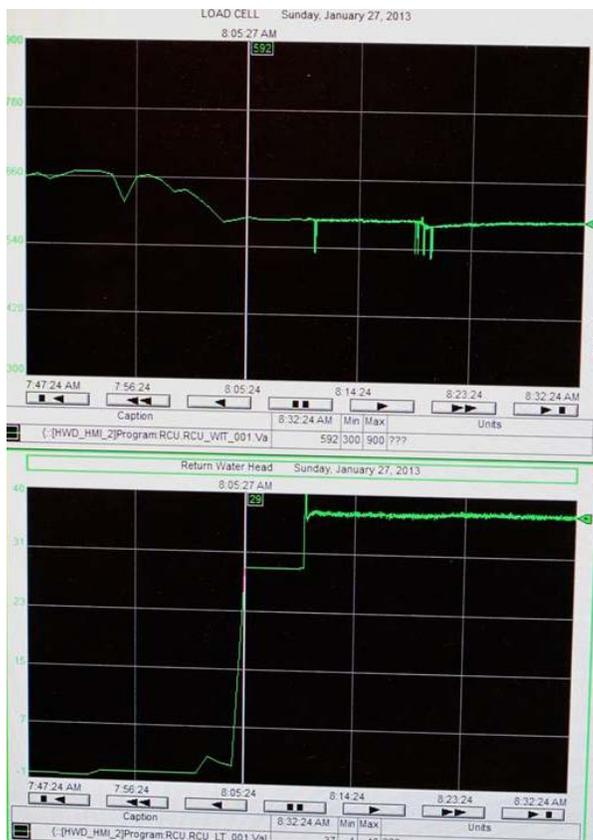
**Figure. Load cell and water level data from drill sensors indicating possible lake entry at 0802 h, 27 January 2013. The vertical white line reveals the temporal region when sensors changed.**
